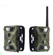
**Needed:** 8xAA alkaline or 8xAA rechargeable batteries, see manual where to fit. important note: you have to select the battery type you choose to use in the menu. you can also choose to use a solar panel. if a solar panel will be used, please make sure there are no batteries in the unit as this will cause permanent damage to the camera!
